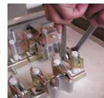
(2) 拧下需更换的硅钼棒夹头螺丝
